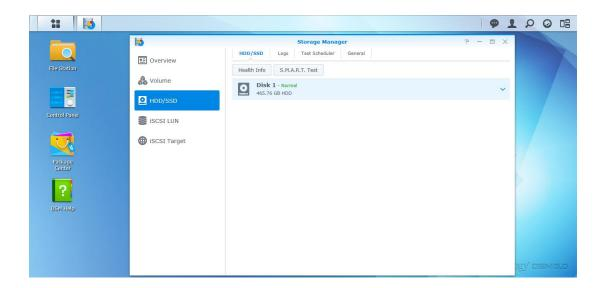
2. DS112j only supports creating one volume (as shown in the figure below) and a volume can only be attached to one IP camera when using NFS mount type. There might be confliction that causes HDD error and video loss if a volume is attached to more than one IP camera.
