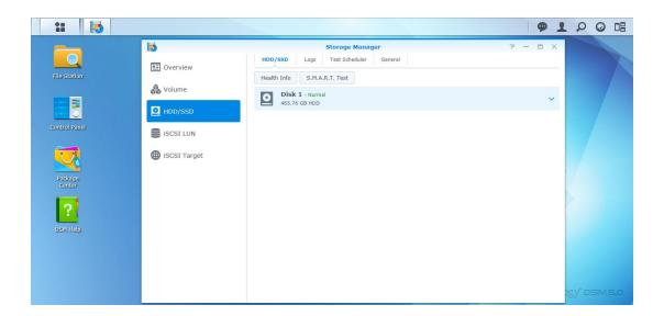
2. DS112j only supports creating one volume (as shown in the figure below). If you want to attach more than one IP camera to a volume, please create multiple shared folders and users on DS112j. Note that quota mode must be enabled on every single user and the total quota size of all users must be smaller than the volume size. After that you should assign each shared folder to each user and then input each shared folder (file path) and user info in the web client of each IP camera.
