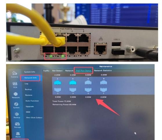
1. Check whether the indicator light of the NVR POE interface is on.
